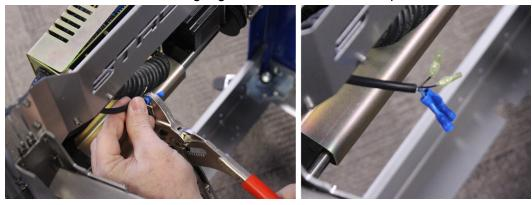
Next, shorten the new heatbed wires leaving approximately 3" (80mm) of wire for splicing. Strip the wires so they will work with the wire connectors.
