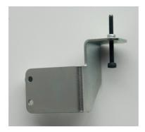
The Z-Assembly Bracket is mounted to the two open mounting holes shown below. To attach the bracket, use the 2.5mm hex wrench and the good pair of pliers to hold the M3 nylon lock nut. Make sure the nuts are tight and the bracket is firmly attached. Any movement in the bracket will affect your bed leveling and subsequently affect your print quality.
