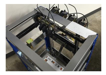
With the template positioned correctly, use a drill hole punch or alternate method to accurately mark the two drill locations.
