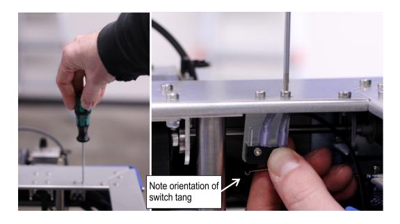
Step 3. Remove the Z-Probe Bracket
