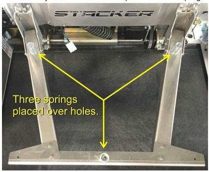
As you lower the bed, the leveling studs drop through the springs and into holes. Once they are all in position, you can attached the nuts from underneath the bed. Tighten the three M3 nylon lock nuts until they compress the springs and are approximately to the middle of the stud.
