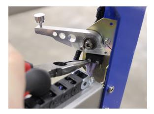
Next, detach the Z-Probe Bracket by removing the two socket head cap screws, nuts and washers using an M3 hex wrench and an 8mm hex nut driver. After the Z-Probe has been removed, reattach the screws and nuts to the same locations on the frame. The two spacer washers are no longer needed.
