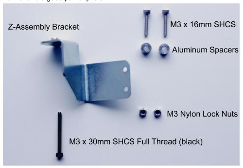
Insert the M3 x 30mm SHCS Full Thread into the Z-Assembly Bracket as shown. The screw should be advanced about half-way through the bracket.
