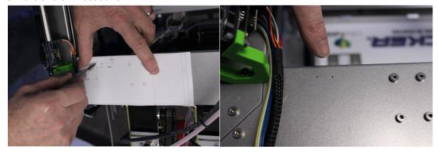
Use a ½" bit to drill the two hole locations you have marked. We recommend applying tape to prevent the drill from scratching the surface of your printer. Also, it is important to use a shop vacuum while drilling to collect the metal debris. *The metal debris created during drilling can cause serious damage to your printer, so be sure to use a vacuum while drilling!*
