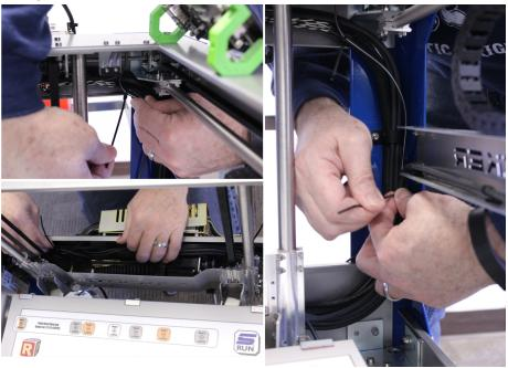
Make sure the wire is zip tied to avoid any moving parts of your printer. Be sure to trim the tails from the zip ties.
