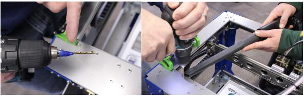
After the two holes have been drilled, use a flathead screwdriver to smooth and remove any metal burrs from the underside the drilled holes.
