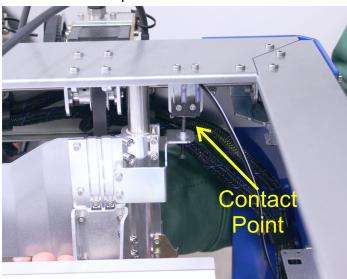
If a print nozzle makes contact with the bed before Z-endstop screw can reach the contact point with the switch, then you should first verify the location of the nuts on the leveling screws. The nuts should be at least midway up the leveling screws to compress the springs slightly.
