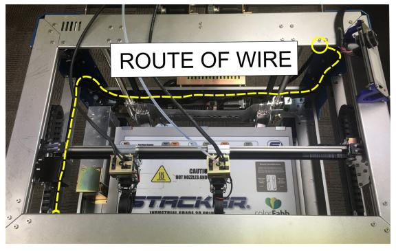
To connect the endstop wires, carefully insert the wires you stripped into the housing and crimp. Polarity is unimportant but both wires must be properly connected for your new end stop to function.
