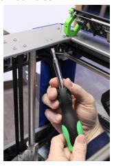
Step 2. Install the New Z-Endstop.
