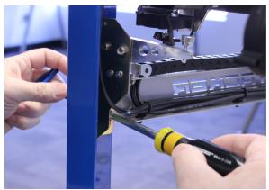
**Step 4. Reconnect the the Endstop Wire**
