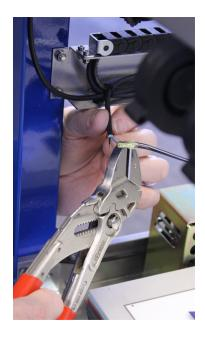
Now that the wire is connected, take up the slack in the wire by using the zip ties to attach the wire to the existing wire bundles.
