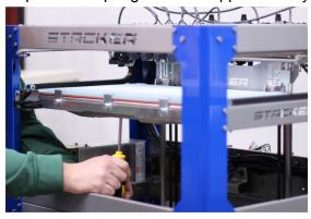
Move to the rear of the printer (or tip a desktop printer on its side) to carefully insert the 18 gauge heat bed wires into the blue crimp connectors and crimp them. Then, insert the two smaller 24 gauge wires to the small yellow wire crimp connectors and crimp these. Again, polarity is unimportant, but the wires must be properly connected for your new heater bed to function properly.
