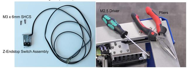
Hold the Endstop Switch as shown below and use the two M3 x 6mm SHCS to attach the switch to the frame through the holes you drilled in Step 1. Note the position of the switch and orientation of the tang in the image below. Run the switch wires toward the wires bundled along the rear interior leg of the frame.
