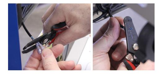
Now, you will need to carefully run the wires from the new Z-Stop Switch Assembly to the wires you just stripped. Run the wire along the current wire bundles. Avoid twisting this endstop wire with the existing wires -- just lay the wire along the route. You will zip tie the wires after the connects are made.
