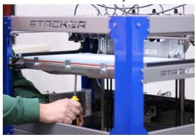
Once the nuts have been removed, the entire bed will lift easily off the printer. When you lift the print bed, the springs will fall from the leveling screws -- be careful to avoid losing these springs, you will need them to install the new bed.
